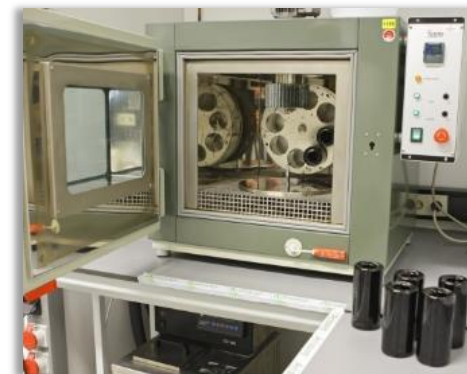
Pressure Aging Vessel 20 h at 100 °C
