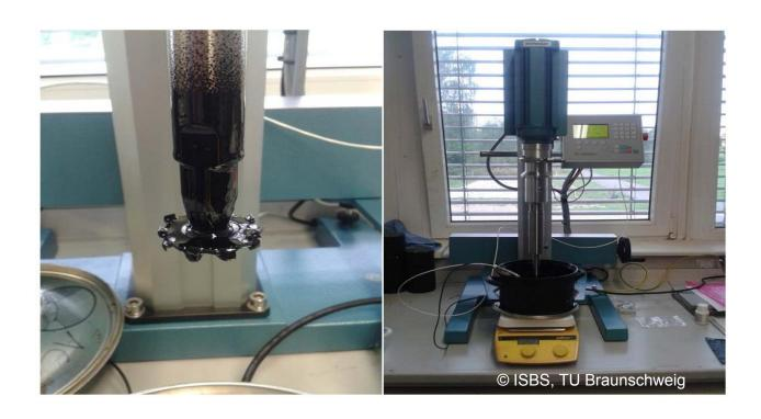
Blending of bitumen and ZycoTherm®: cowles agitator (left) and mixer used (right)
