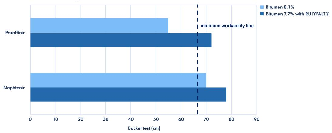
Both Naphtenic and Paraffinic bitumen treated with Rulyfalt® Technology show an improved workability at 200°C with reduced %Bitumen
