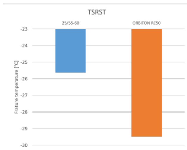
Figure 7. Fracture temperature results acc. to EN 12697-46 [source: ORLEN Asphalt]
